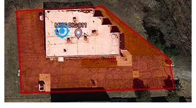
polygon is transmitted on the MISS DIG 811 ticket to the facility owners. The polygon reflects the area the excavator has designated to MISS DIG 811 as the excavation/blasting area to be located and marked. Positive Responses provided are for the entire area covered under the polygon associated with the ticket.
